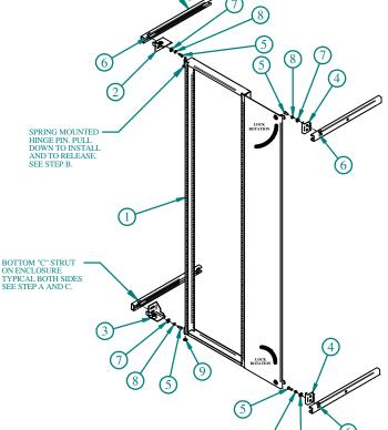
NOTE: MOUNTING HOLES IN THE SIDES OF THE BRACKETS USED IN ILLUSTRATION ARE FOR C2 AND C3 SERIES. USE THE OTHER MOUNTING HOLES IN SIDES OF BRACKETS FOR THE IME AND 1418FS SERIES.
