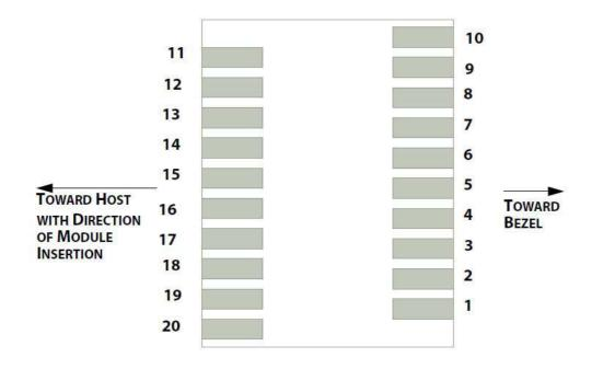
Figure: Module Interface to Host
