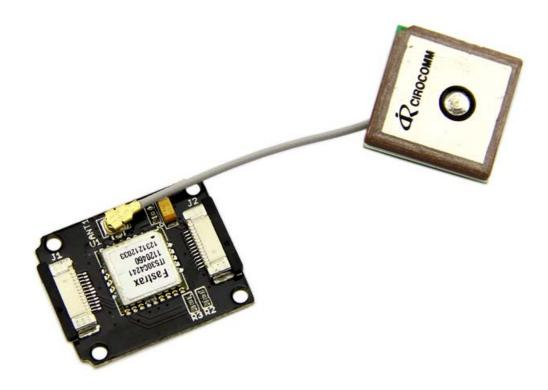
Xadow GPS is an OEM GNSS receiver module, including the Fastrax IT530M and a tiny 12mm squared ceramic patch antenna. The low power module outputs a series of standard NMEA format data which provides position, satellite information and time, etc. This module can be easily connected directly to Xadow Main board to display and record the above-mentioned information. It features acquisition and tracking capability of weak signals, making it a great choice for navigation projects.
