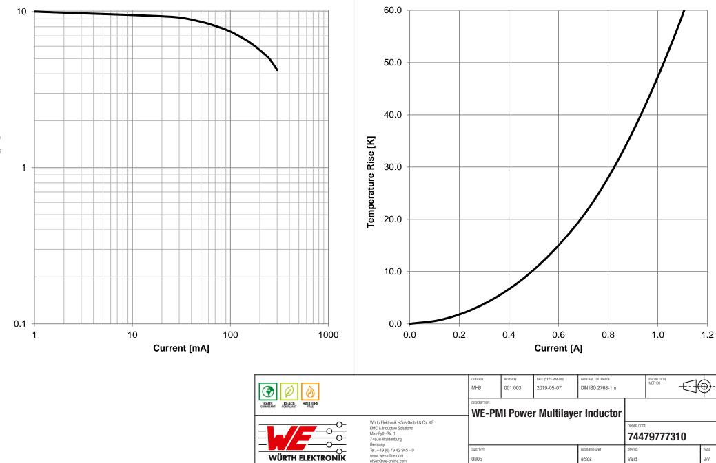
**Typical Temperature Rise vs. Current Characteristics:**
