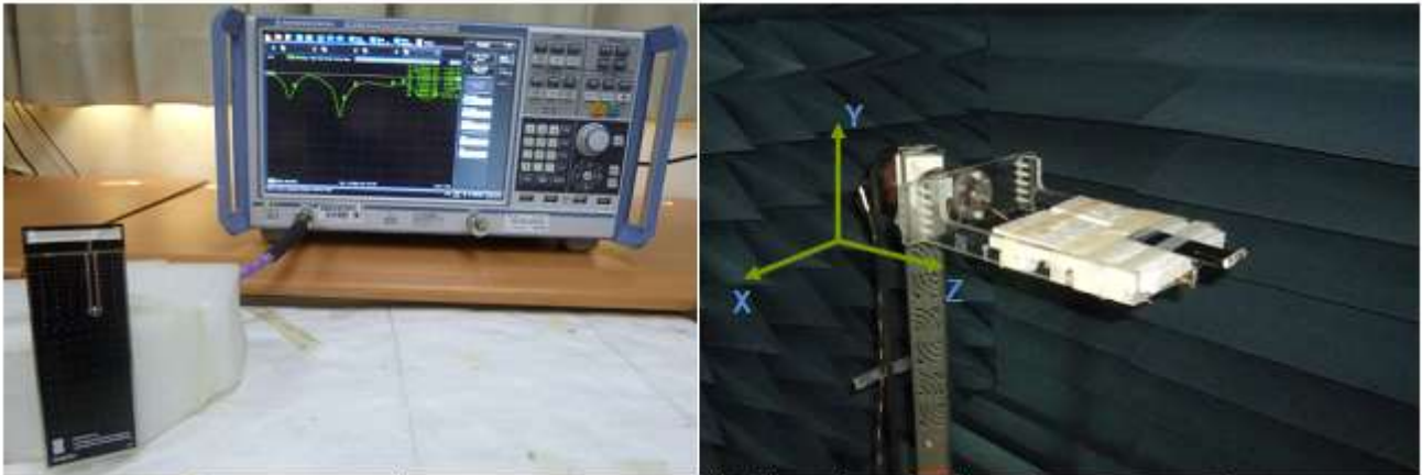
Impedance measurements (left hand) and peak gain, average gain, efficiency and radiation pattern measurements (right hand)
