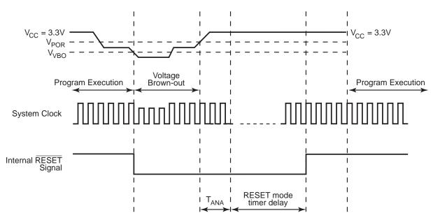
Figure 4. Voltage Brownout Reset Operation
