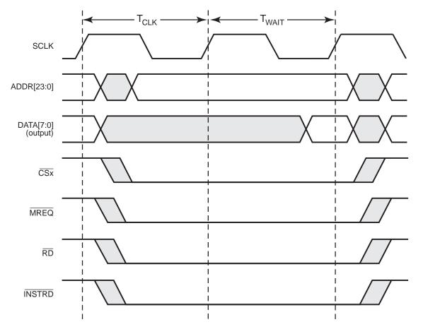
Figure 9. Example: Wait State Read Operation
