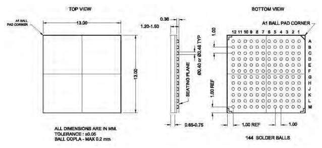
Figure 77 displays the 144-pin chip array ball grid array (BGA) package for the eZ80F91 device.
