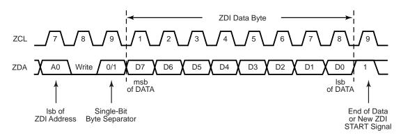
Figure 53. ZDI Single-Byte Data Write Timing
