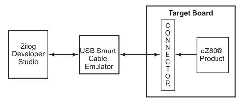
Figure 48. Typical ZDI Debug Setup
