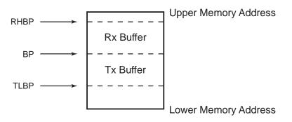
Figure 60. Internal Ethernet Shared Memory
