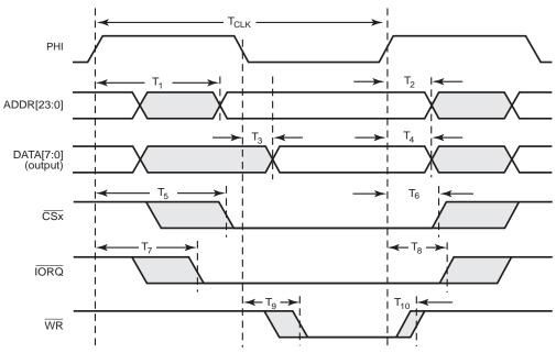
Figure 71. External I/O Write Timing
