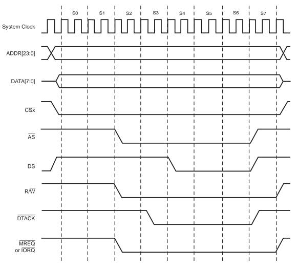
Figure 19. Example: Motorola Bus Mode Write Timing
