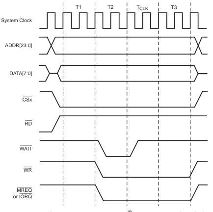
Figure 11. Example: Z80<sup>®</sup> Bus Mode Write Timing
