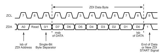
Figure 55. ZDI Single-Byte Data Read Timing
