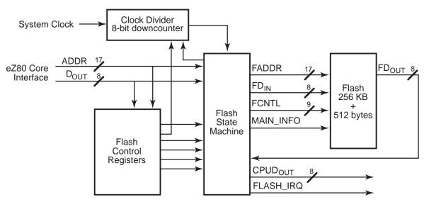
Figure 24. Flash Memory Block Diagram
