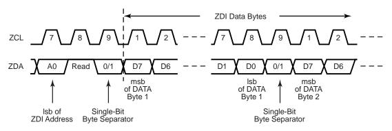
Figure 56. ZDI Block Data Read Timing
