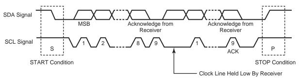
Figure 45. I<sup>2</sup>C Frame Structure
