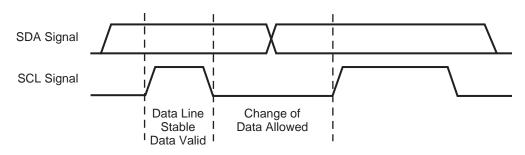
Figure 43. I<sup>2</sup>C Clock and Data Relationship
