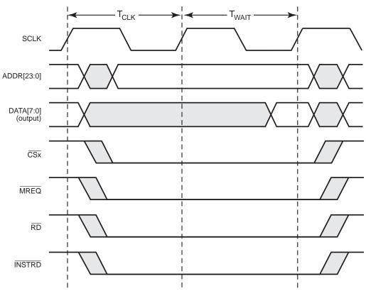
Figure 72. Wait State Timing for Read Operations
