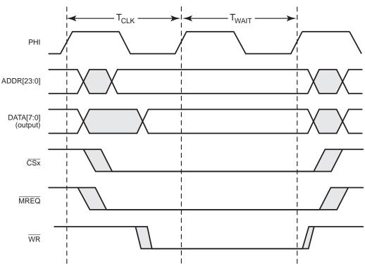
Figure 73. Wait State Timing for Write Operations
