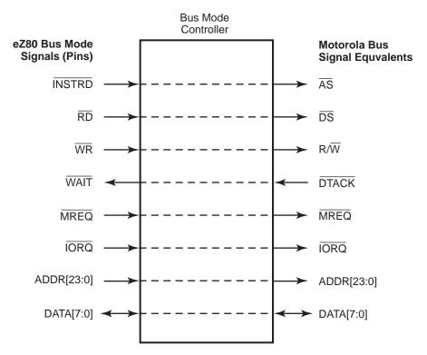
Figure 17. Motorola Bus Mode Signal and Pin Mapping
