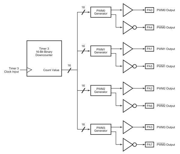
Figure 30. Multi-PWM Simplified Block Diagram
