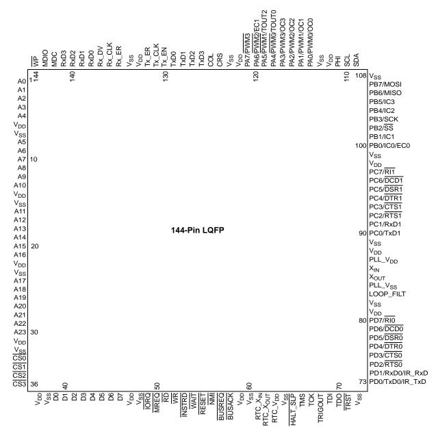
Figure 2 displays the pin layout of the eZ80F91 device in the 144-pin LQFP package.
