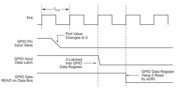
Figure 74. Port Input Sample Timing
