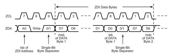
Figure 54. ZDI Block Data Write Timing
