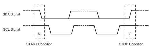
Figure 44. START and STOP Conditions In I<sup>2</sup>C Protocol
