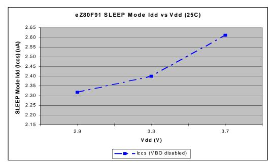
Figure 67.  $I_{\text{CC}}$  vs. Vdd During SLEEP Mode
