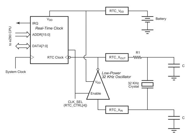
Figure 35. Real-Time Clock and 32 kHz Oscillator Block Diagram
