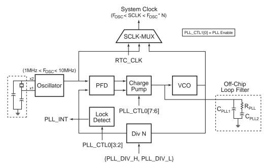
Figure 57. Phase-Locked Loop Block Diagram
