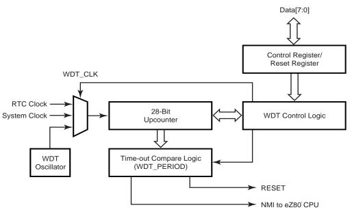
Figure 25. Watchdog Timer Block Diagram
