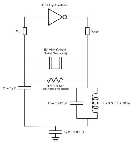
Figure 63. Recommended Crystal Oscillator Configuration—50 MHz Operation
