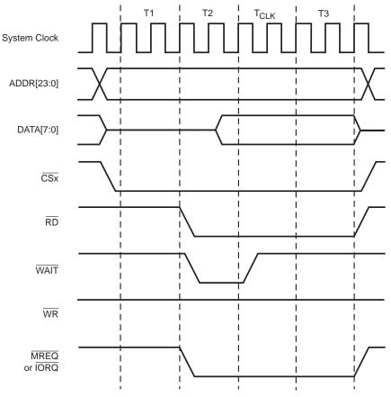
Figure 10. Example: Z80 Bus Mode Read Timing
