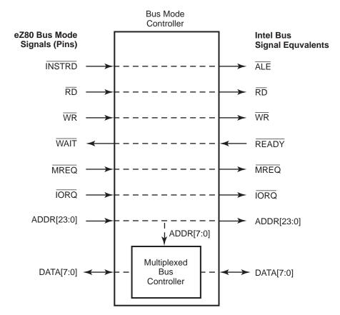
Figure 12. Intel Bus Mode Signal and Pin Mapping
