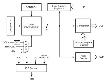
Figure 26. Programmable Reload Timer Block Diagram
