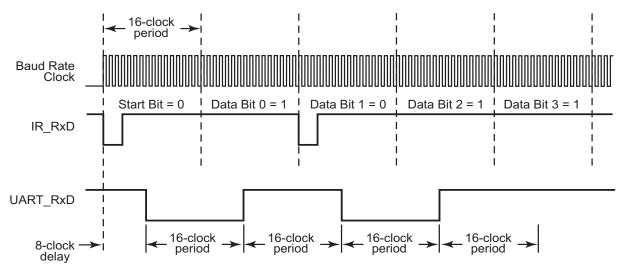
period. If the data to be received is a logical 0, a delayed Low (0) pulse is output on RxD. Data transmission is displayed in Figure 39.
