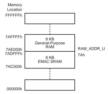
Figure 22. Example: eZ80F91 On-Chip RAM Memory Addressing
