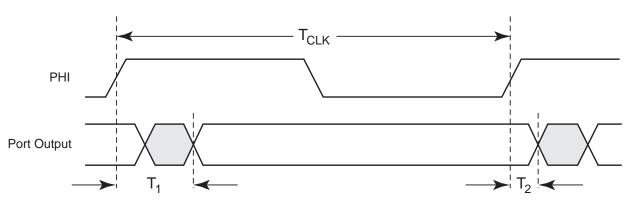
Figure 75. GPIO Port Output Timing
