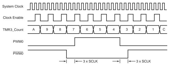
Figure 34. PWM Nonoverlapping Output Delay
