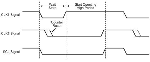
Figure 47. Clock Synchronization In I<sup>2</sup>C Protocol
