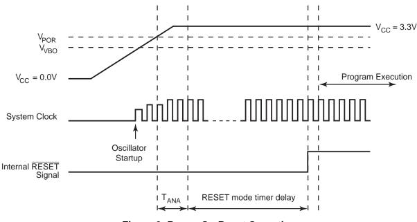
Figure 3. Power-On Reset Operation
