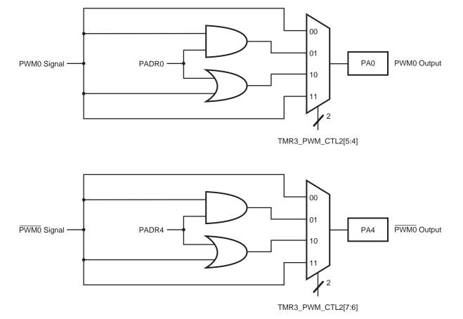
Figure 33. PWM AND/OR Gating Functional Diagram
