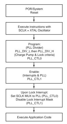
Figure 58. Normal PLL Programming Flow
