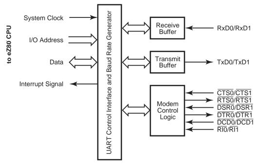
Figure 36. UART Block Diagram
