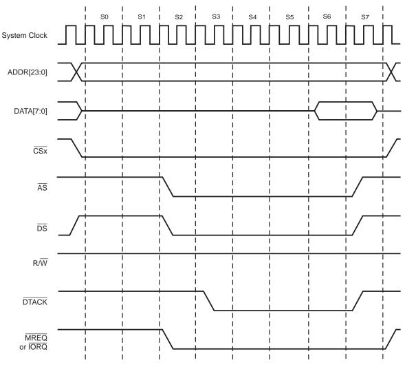
Figure 18. Example: Motorola Bus Mode Read Timing
