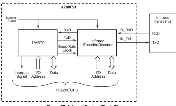
Figure 37. Infrared System Block Diagram
