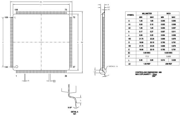
Figure 76. 144-Lead Plastic Low-Profile Quad Flat Package (LQFP)
