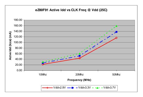
Figure 65.  $I_{\text{CC}}$  vs. System Clock Frequency During ACTIVE Mode
