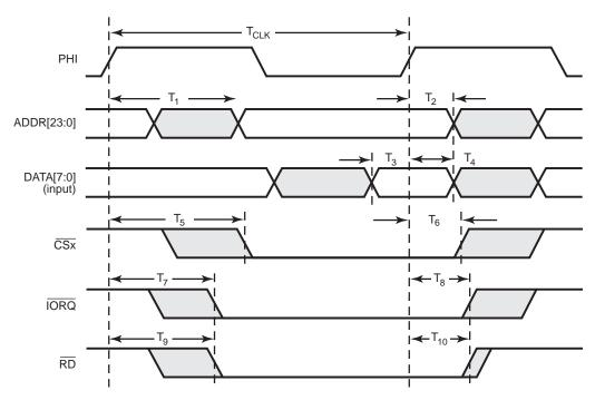
Figure 70. External I/O Read Timing
