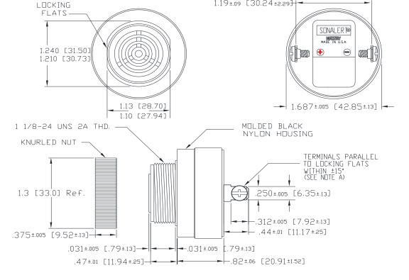
NOTE A: TERMINALS-.032 BRASS TIN PLATED, TAPPED FOR #6-32 SCREW. TWO #6-32 NICKEL PLATED BRASS SCREWS INCLUDED. WILL ACCEPT 1/4" QUICK CONNECT. NOTE B: MOUNTING- REMOVE BLACK PLASTIC NUT AND INSERT THREADED FRONT THROUGH 1.25" HOLE PUNCHED IN PANEL, IF DRIENTATION IS NEEDED, NOTE LOCKING FLATS ON DRAWING. SCREW NUT BACK ON. DO NOT OVERTIGHTEN.
