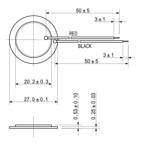
1) Metal :Brass 2) Ceramic :KPM-31 3) Electrode :Silver 4) Leads :AWG-32 5) Unit :mm
