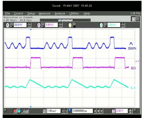
Figure 23. Switcher Operation – DCM Mode
