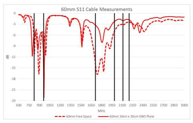
Taoglas recommend a minimum cable length of 60mm for this antenna when used on a ground plane to achieve an efficiency of greater than 20%.
