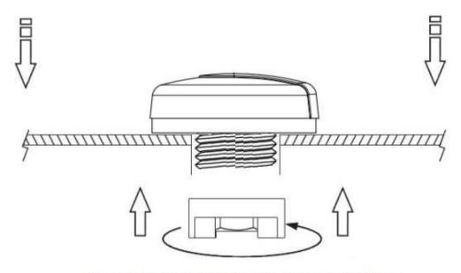
Recommended torque for Mounting is 3.92N·m Maximum torque for Mounting is 4.9N·m
