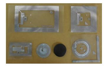
The Tag-it HF-I Plus Transponder Inlay family of Texas Instruments RFID is based on the ISO/IEC 15693 standard for contactless integrated circuit cards (vicinity cards) and ISO/IEC 18000-3 standard for item management.
