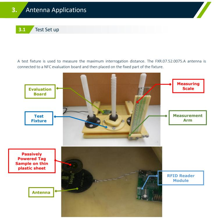
The test sample is placed on a thin sheet of plastic connected to the movable part of the fixture. Then the distance is carefully adjusted until the reader can no longer read the sample, thus the maximum interrogation distance is displayed in the ruler.
