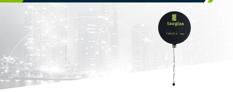
The FXR.07.52.0075X.A is a circular, flexible, NFC (Near Field Communications) antenna for use in mobile devices and other applications such as keycards, payment systems, and boarding passes. The design provides a flexible NFC antenna with 75mm twisted pair 28AWG cable that can be adhered to the plastic enclosure of the device for ease of installation and work with specific 13.56MHz RFID and NFC chips which need to connect via JST ACH connector.
