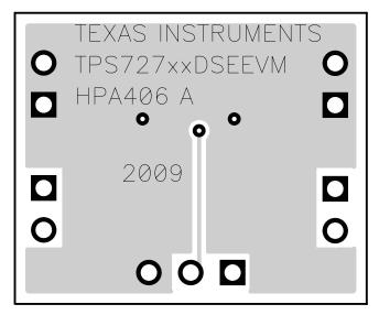
Figure 4. Bottom Layer Assembly
