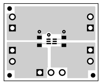
Figure 2. Top Layer Routing
