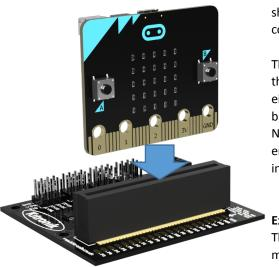
Inserting a BBC micro:bit: To use the servo driver board the BBC micro:bit should be inserted firmly into the connector as shown left.
