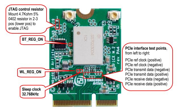
Figure 3 – 1CX M.2 Module Test Points and JTAG Control Resistor
