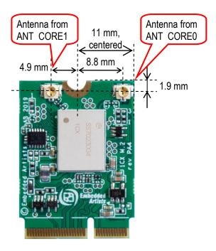
Figure 1 - M.2 Module Antenna Connector Measurements
