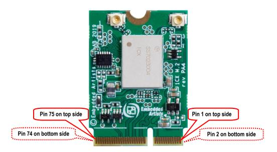
Figure 2 - M.2 Module Pin Numbering
