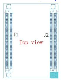
Figure 1-7 Expansion Connectors of MYC-C7Z015
