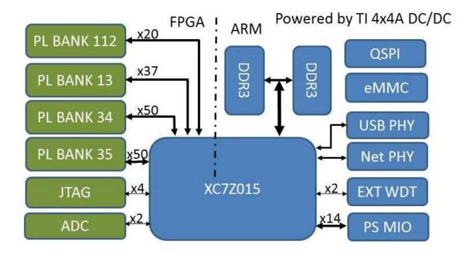
Figure 1-5 MYC-C7Z015 Function Block Diagram
