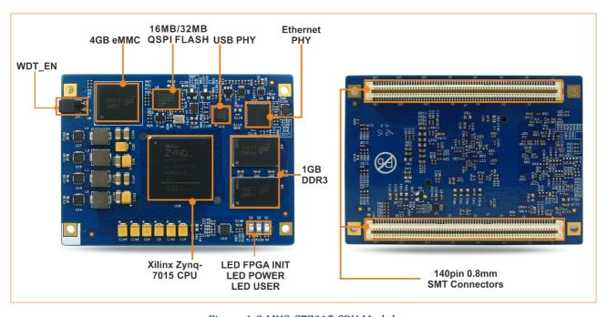
Figure 1-2 MYC-C7Z015 CPU Module
