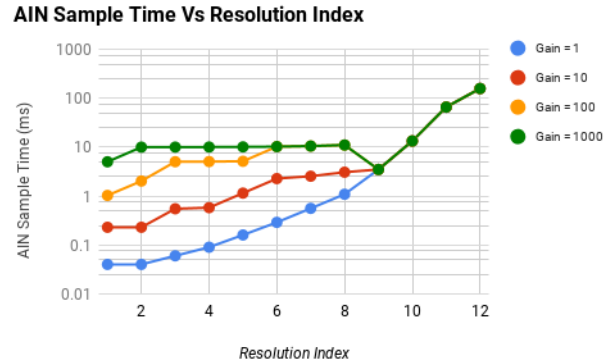
Figure A.3.1.4. T7 AIN sample times for analog inputs over various gains resolution index settings.
