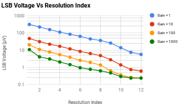
Figure A.3.1.3. T7 analog input LSB voltage over various gains and resolution index settings.
