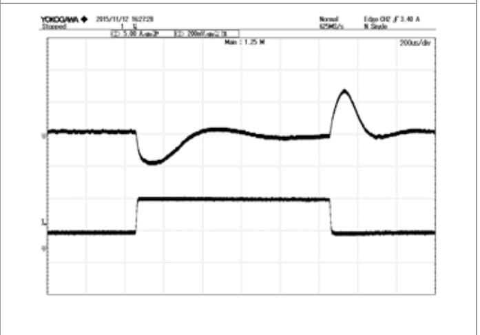
Figure 4: Dynamic response to load step 25%~75% with 0.1A/uS slew rate at 220Vac
