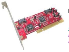
**TR-822** SATA RAID 2 Ports Low Profile PCI Host Adapter Low Profile PCI 1.5Gbps Native SATA internal 2Ports with RAID 0, RAID 1 support!
