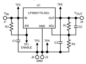
Figure 1. Schematic for Basic Application Circuit
