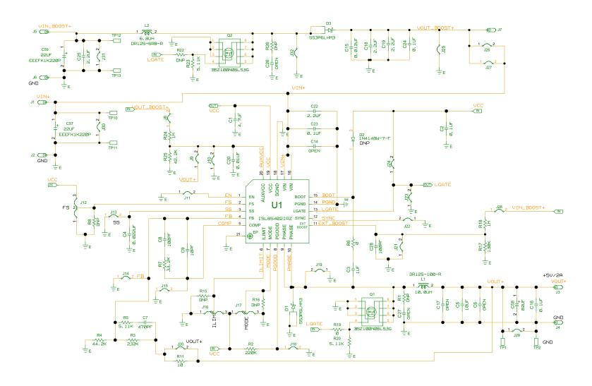
FIGURE 2. ISL85402EVAL1Z EVALUATION BOARD SCHEMATIC
