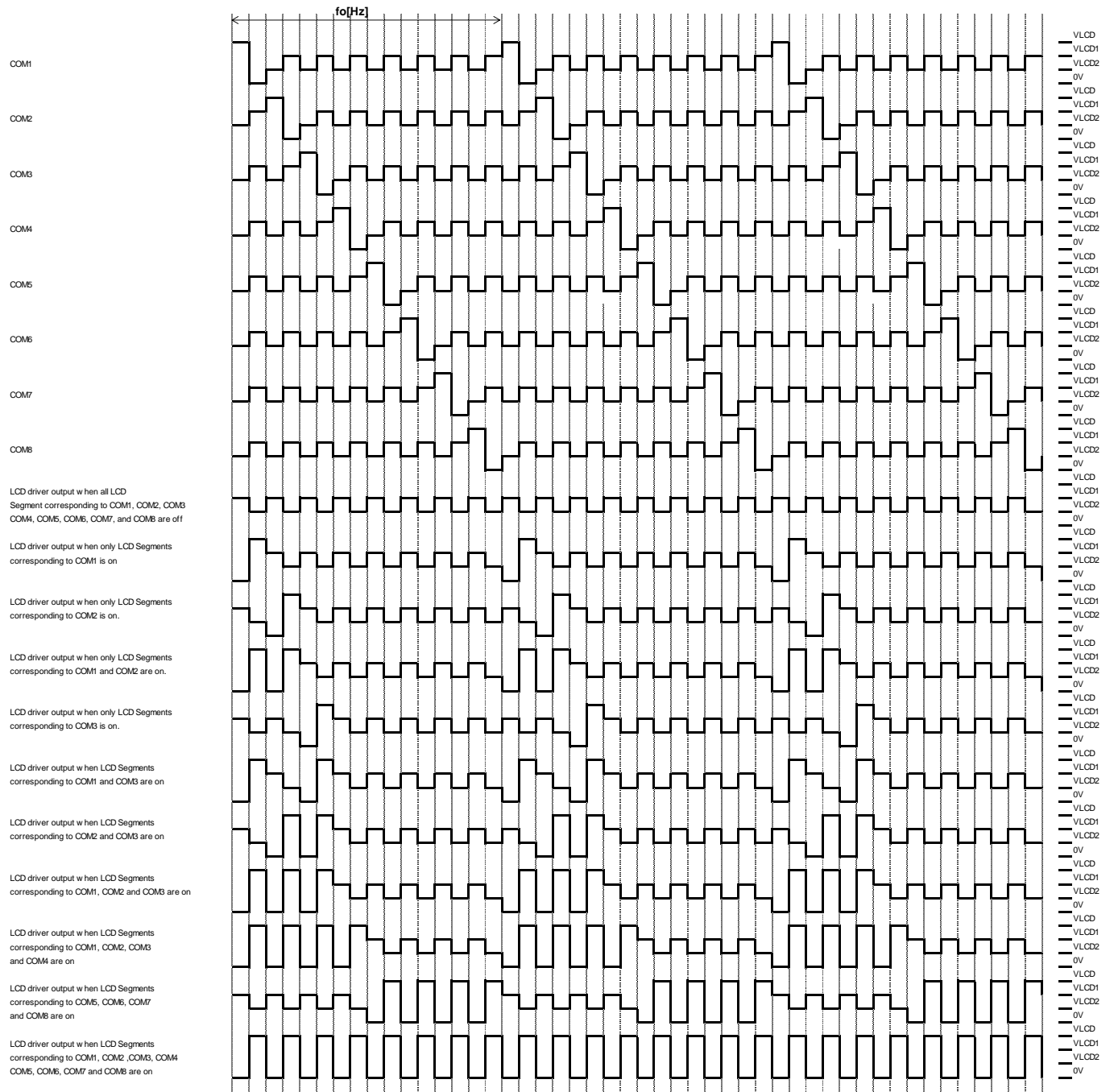
Figure 29. LCD Waveform (Line Inversion, 1/8 DUTY, 1/3 BIAS)
