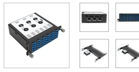
Singlemode fiber cassette installs in Tripp Lite N484-Series chassis to connect 12 duplex LC fiber cables with three 8-fiber MTP/MPO (APC) connections in high-density network applications.
