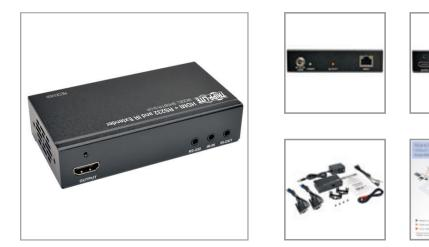
Works with a Tripp Lite HDBaseT matrix transmitter to extend uncompressed HDMI video and audio, RS-232 serial and IR remote control signals over a Cat5e/6/6a cable up to 328 ft. to a projector, monitor or television.
