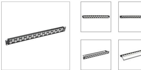
Feed-through patch panel with staggered RJ45 jacks manages and organizes Cat6a input and output cable connections and reduces crosstalk in your high-density 10 Gbps Ethernet network. No 110 punchdown termination required.
