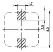
no sensitive traces underneath the component
