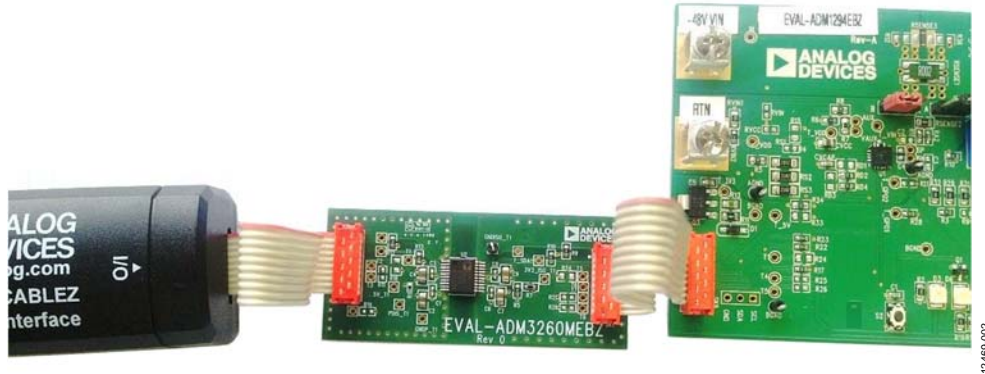
Figure 2. Board Connection Example
