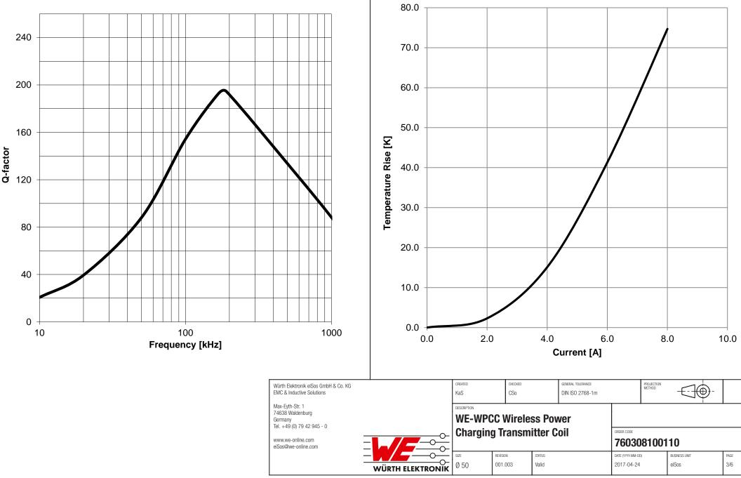
**Typical Temperature Rise vs. Current Characteristics:**
