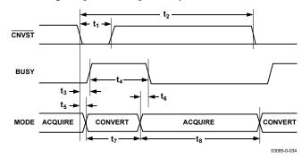
Figure 33. Basic Conversion Timing
