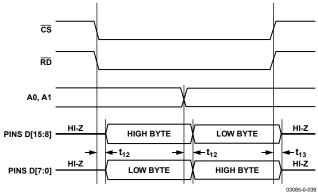
Figure 38. 8-Bit and 16-Bit Parallel Interface
