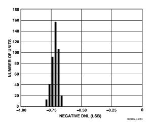
Figure 13. Typical Negative DNL Distribution (424 Units)
