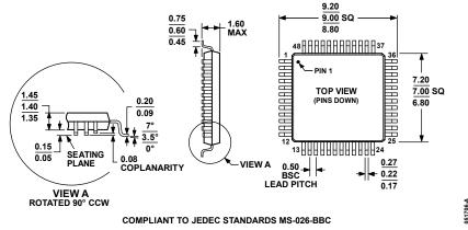
Figure 45. 48-Lead Low Profile Quad Flat Package [LQFP] (ST-48)
