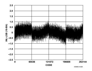
Figure 6. Integral Nonlinearity vs. Code
