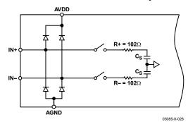
Figure 27. Simplified Analog Input
