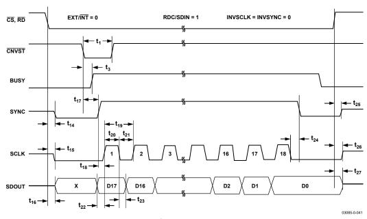
Figure 40. Master Serial Data Timing for Reading (Read Previous Conversion during Convert)
