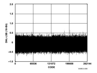
Figure 9. Differential Nonlinearity vs. Code
