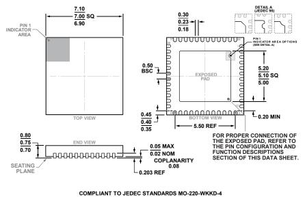
Figure 46. 48-Lead Lead Frame Chip Scale Package [LFCSP] 7 mm × 7 mm Body and 0.75 mm Package Height (CP-48-4) Dimensions shown in millimeters
