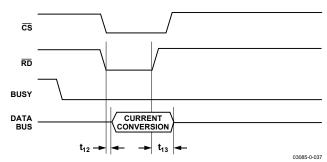
Figure 36. Slave Parallel Data Timing for Reading (Read after Convert)
