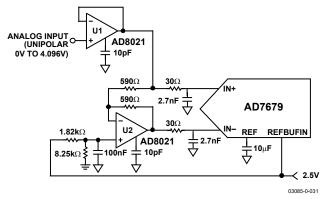
Figure 30. Single-Ended-to-Differential Driver Circuit (Internal Reference Buffer Used)
