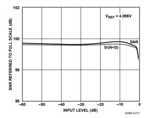
Figure 17. SNR and S/(N+D) vs. Input Level
