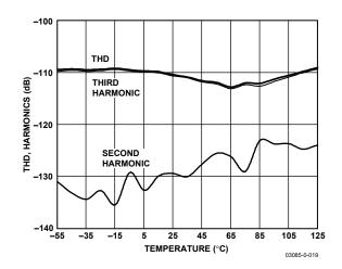
Figure 19. THD and Harmonics vs. Temperature
