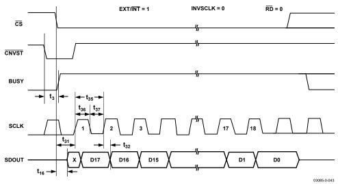
Figure 42. Slave Serial Data Timing for Reading (Read Previous Conversion during Convert)
