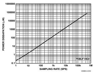
Figure 32. Power Dissipation vs. Sample Rate
