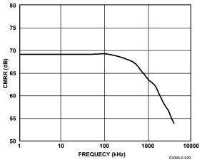
Figure 28. Analog Input CMRR vs. Frequency
