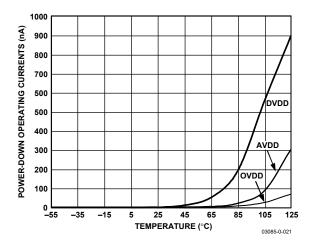
Figure 21. Power-Down Operating Currents vs. Temperature
