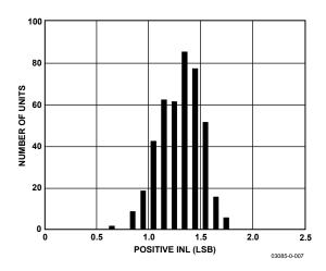
Figure 8. Typical Positive INL Distribution (424 Units)
