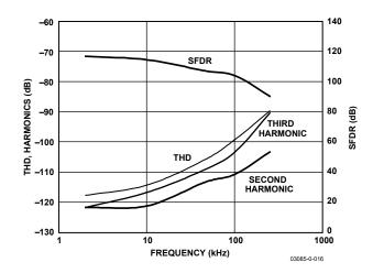
Figure 16. THD, SFDR, and Harmonics vs. Frequency
