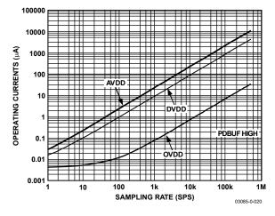
Figure 20. Operating Current vs. Sampling Rate
