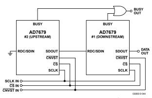
Figure 43. Two AD7679s in a Daisy-Chain Configuration
