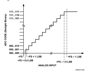
Figure 25. ADC Ideal Transfer Function
