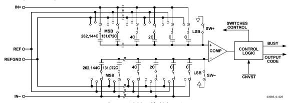
Figure 24. ADC Simplified Schematic
