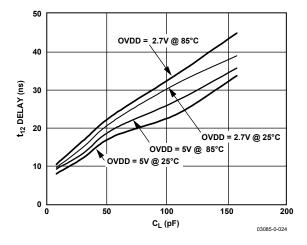
Figure 23. Typical Delay vs. Load Capacitance CL
