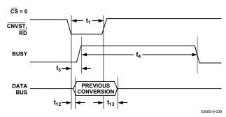
Figure 37. Slave Parallel Data Timing for Reading (Read during Convert)
