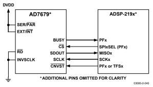
Figure 44. Interfacing the AD7679 to an SPI Interface
