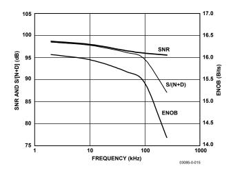
Figure 15. SNR, S/(N+D), and ENOB vs. Frequency
