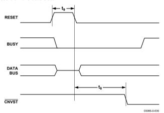
Figure 34. RESET Timing
