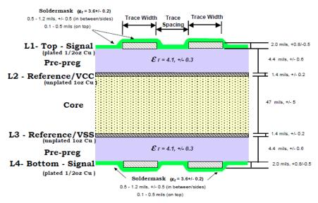
Figure 7-11 4-Layer PCB Stack-up Example
