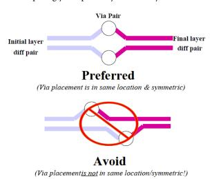
Figure 7-18 Layout Guidance of Stitching Via
