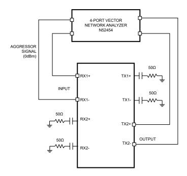
Figure 6-3 Channel-Isolation Test Configuration
