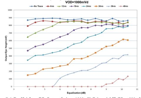
Figure 7-6 Eye Height vs EQ, Output Swing =1000mV, Gain=+2.5dB (Vin =800mVdiff)
