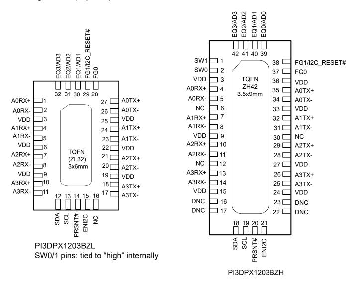
Figure 3-1 32/42-pin package pin-out
