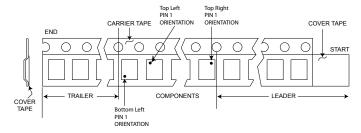
Figure 8-6 Tape Leader and Trailer pin 1 Orientations
