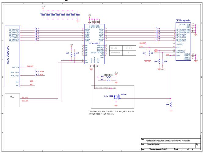
Figure 7-2 DP Source Application in Pin Mode
