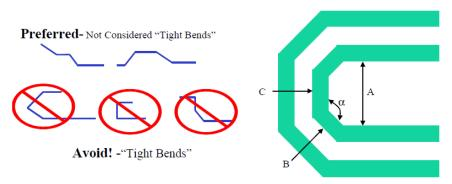
Figure 7-15 Layout Guidance of Bends
