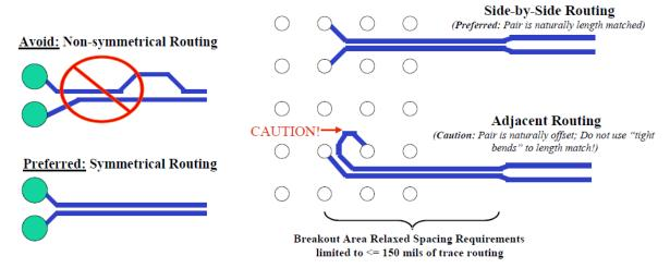
Figure 7-14 Layout Guidance of Matched Differential Pair
