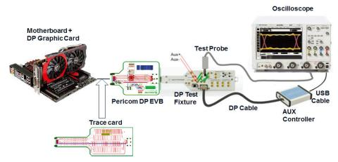
Figure 7-19 Displayport test set-up
