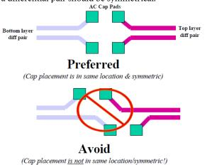
Figure 7-17 Layout Guidance of Series Component
