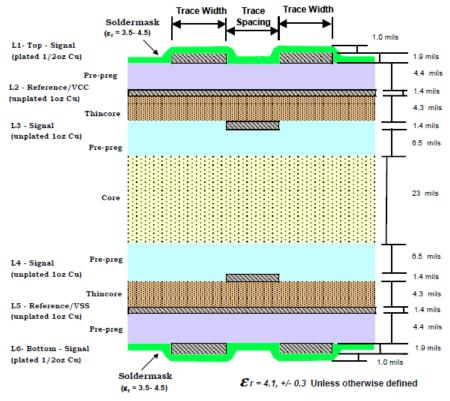
Figure 7-12 6-Layer PCB Stack-up Example
