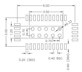
Figure 8-2 32-contact TQFN (ZL32) Package Mechanical Drawing with Ground Via Information
