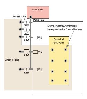
Figure 7-9 Decoupling Capacitor Placement Diagram
