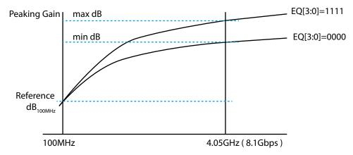
Figure 6-6 Definition of Peaking Gain relative to 100 MHz, 100 mVp-p sine wave input
