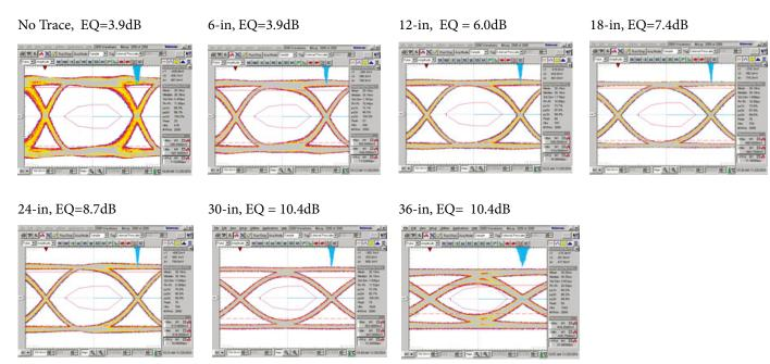
Figure 7-7 Output Eye Diagram at FG 0.5dB
