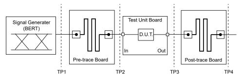
Figure 6-2 AC Electrical Measurement Test Setup
