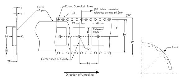
Figure 8-7 Standard Embossed Carrier Tape Dimensions
