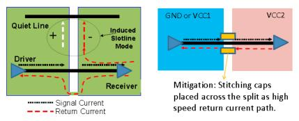
Figure 7-13 Stitching Capacitor Placement
