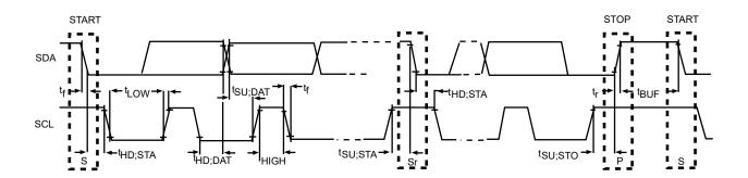
Figure 6-7 I<sup>2</sup>C Timing Diagram
