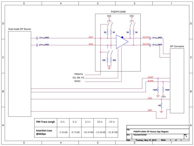
Figure 7-1 Source side DP Redriver Connection Diagram
