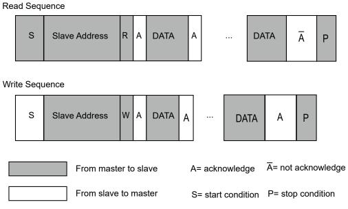
Figure 5-2 I2C Read / Write Timing Sequence
