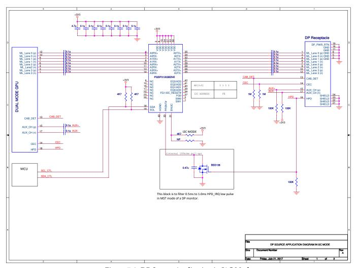
Figure 7-3 DP Source Application in I2C Mode
