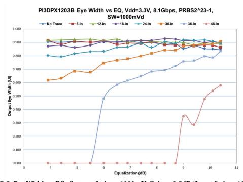
Figure 7-5 Eye Width vs EQ, Output\_Swing =1000mV, Gain=+0.5dB (Input Swing=1000mVd) PI3DPX1203B Eye Height vs EQ, Vdd=3.3V, 8.1Gbps, PRBS2^23-1,
