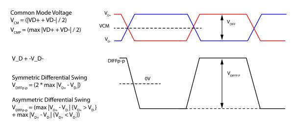
Figure 6-5 Definition of Differential Voltage and Differential Voltage Peak-to-Peak
