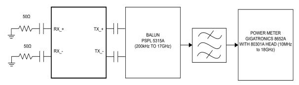
Figure 6-4 Noise Test Configuration
