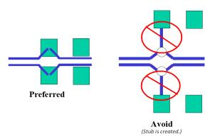
Figure 7-16 Layout Guidance of Shunt Component
