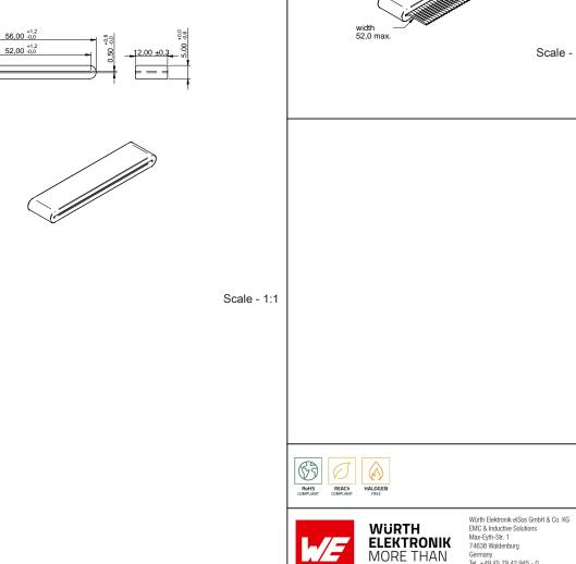
**Operating Temperature** -25 up to +125 °C Storage Conditions (in original < 40 °C; < 75 % RH packaging) Test conditions of Electrical Properties: +20 °C, 33 % RH if not specified differently CHECKED REVISION DATE (YYYY-MM-DD) GENERAL TOLERANCE PROJECTION METHOD JaH 004.007 2022-01-03 DIN ISO 2768-1m DESCRIPTION **WE-FLAT Flat Ferrite Core** ORDER CODE 7427807 STATUS Tel. +49 (0) 79 42 945 - 0 BUSINESS UNIT PAGE YOU EXPECT www.we-online.com eiSos Valid 1/6 eiSos@we-online.com
