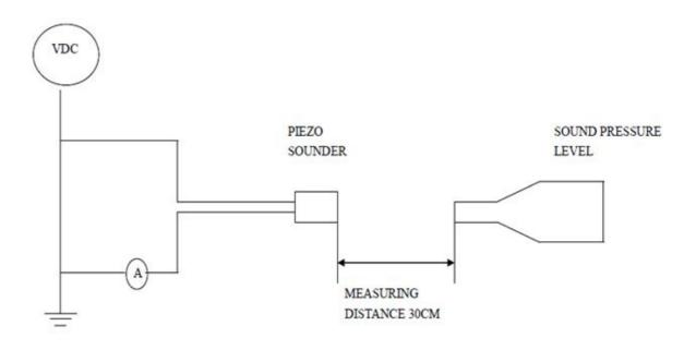
MIC: S.P.L meter TES1351B or equivalent
