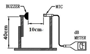
Mic: RION S.P.L meter UC30 or equivalent S.G: Hewlett Packard 33120A Function Generator or equivalent
