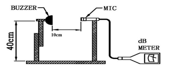
MIC: S.P.LmeterTES1351B or equivalent S.G: Hewlett Packard EE1641B Function Generator or equivalent
