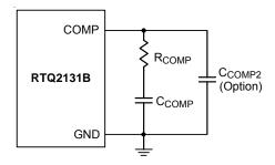
Figure 6. External Compensation Components
