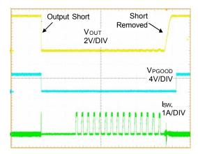
Figure 3. Short Circuit Protection and Recovery
