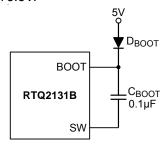
Figure 8. External Bootstrap Diode
