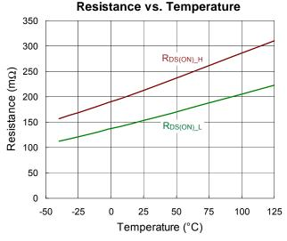
Figure 14. RTQ2131B R<sub>DS(ON)</sub> vs. Temperature
