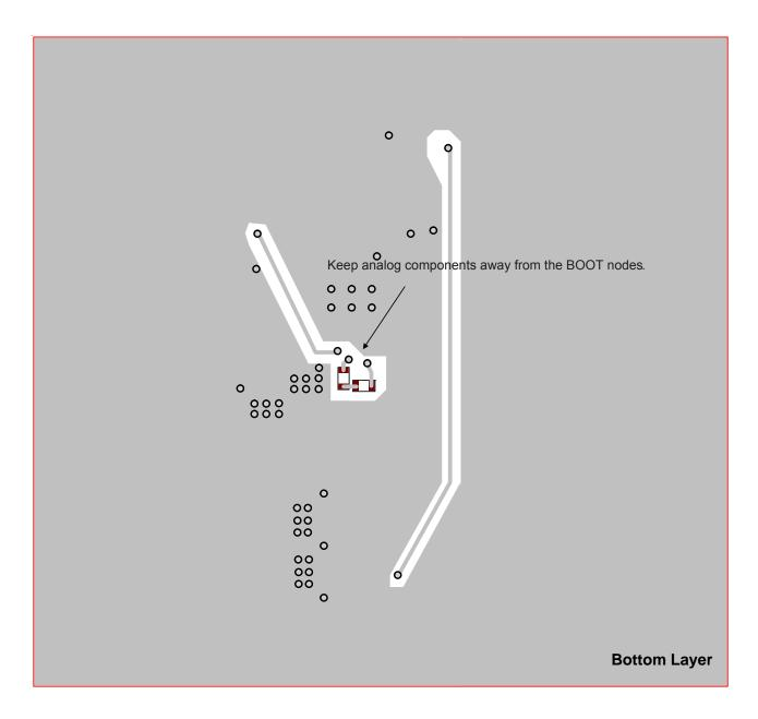
Figure 18. Layout Guide (Bottom Layer)
