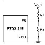
Figure 5. Output Voltage Setting
