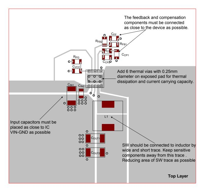
Figure 15. Layout Guide (Top Layer)
