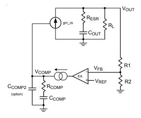
Figure 7. Simplified Equivalent Circuit of Buck with PCMC
