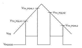
Figure 2. The Logic of PGOOD
