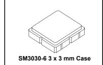
The RO3156E is a true one-port, surface-acoustic-wave (SAW) resonator in a surface-mount ceramic case. It provides reliable, fundamental-mode, quartz frequency stabilization of fixed-frequency transmitters operating at 868.95 MHz.This SAW is designed specifically for SRD remote control and wireless security transmitters operating under ETSI EN 300 220.
