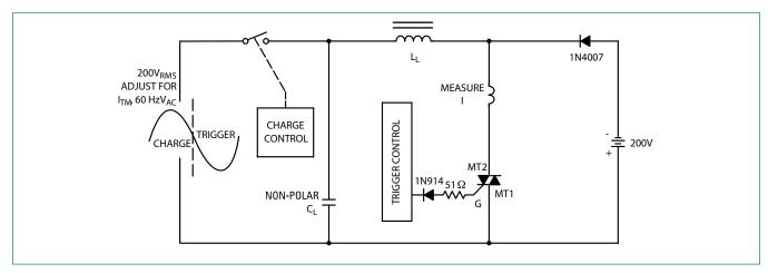
**Note:** Component values are for verification of rated (di/dt)<sub>c</sub>. See AN1048 for additional information
