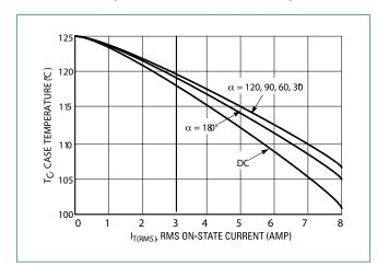
Figure 3. On-State Characteristics
