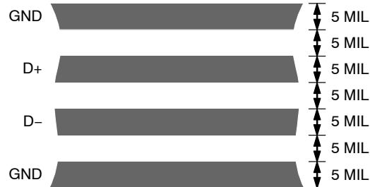
Figure 28. Arrangement of Signal Tracks
