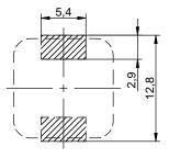
no sensitive traces underneath the component
