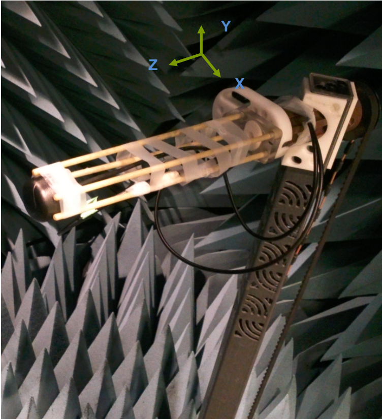
Figure 2. Peak gain, efficiency and radiation pattern measurements
