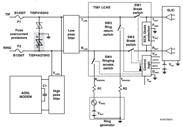
Figure 9. ADSL IVD using Common Protection
