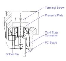
of K7075P, K70100P and K70150P and plug directly onto the board(s). *Solder Pins* are also provided in these enclosures for terminal-to-board connections when mounting an additional board directly behind the front cover. A *Wire Jumper* can be soldered to these pins as well.
