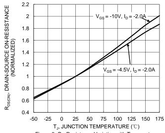
Figure 6. On-Resistance Variation with Temperature
