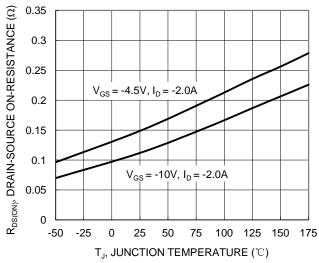
Figure 7. On-Resistance Variation with Temperature
