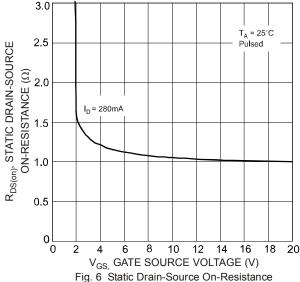
rig. 6 Static Drain-Source On-Resistance vs. Gate-Source Voltage
