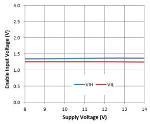
Fig 22. Enable Input Voltage vs. Supply Voltage
