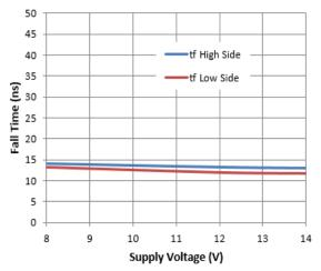
Figure 10. Fall Time vs. Supply Voltage
