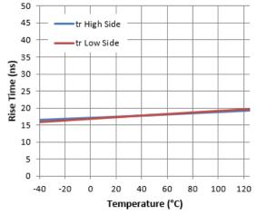
Figure 9. Rise Time vs. Temperature
