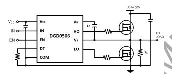
Figure 29. Inrush current is greatly limited by precharging the boost-strap Capacitor through Rs
