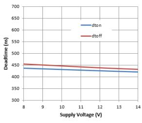
Figure 24. Deadtime vs. Supply Voltage
