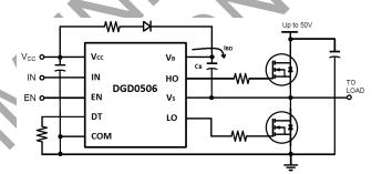
Figure 30. Current into the boost-strap capacitance is shared between the external diode and the internal Diode
