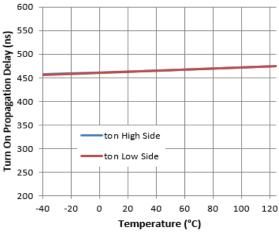
Figure 5. Turn-on Propagation Delay vs. Temperature
