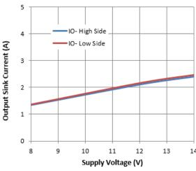
Figure 18. Output Sink Current vs. Supply Voltage
