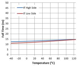
Figure 11. Fall Time vs. Temperature
