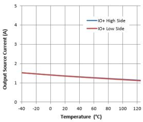
Figure 17. Output Source Current vs. Temperature
