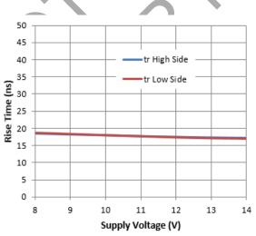
Figure 8. Rise Time vs. Supply Voltage
