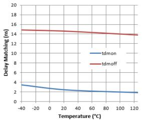
Figure 15. Delay Matching vs. Temperature
