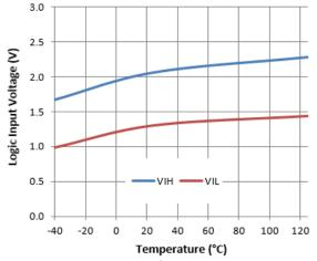
Fig 21. Logic Input Voltage vs. Temperature
