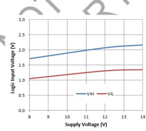
Fig 20. Logic Input Voltage vs. Supply Voltage
