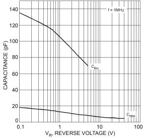
Fig. 6 Typical Capacitance Characteristics
