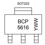
BCP 5616 = Product Type Marking Code YWW = Date Code Marking Y or  $\overline{Y}$  = Last Digit of Year (ex: 0 = 2020) WW or  $\overline{W}W$  = Week Code (01~53)
