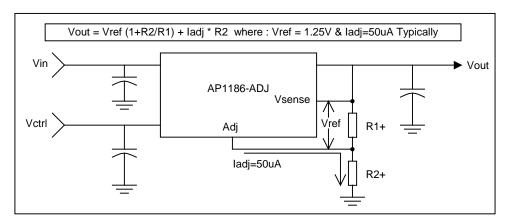
The AP1186-ADJ keeps a constant 1.25V between the Vsense pin and the Adj pin. By placing a resistor R1 across these two pins and connecting the Vsense and Vout pin together, a constant current flows through R1, adding to the ladj current and into the R2 resistor producing a voltage equal to the (1.25/R1)\*R2 + ladj\*R2. This voltage is then added to the 1.25V to set the output voltage. This is summarized in the above equation.
