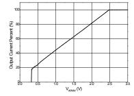
Figure 5. Analog Dimming Curve
