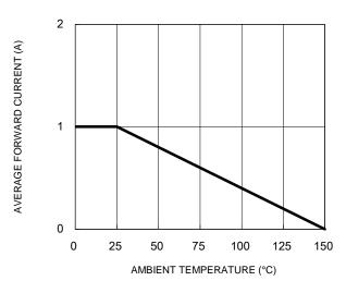
Fig.1 Forward Current Derating Curve
