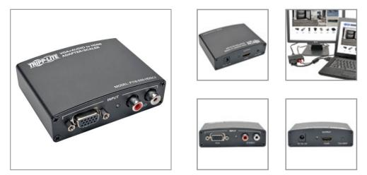
Converts and upscales analog VGA video and RCA stereo audio for display on an HDMI monitor without having to upgrade your source equipment. Ideal for home audio/video setups, media presentations and digital signage.
