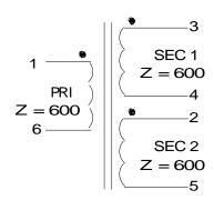
BOTH SECONDARIES MUST BE LOADED FOR IMPEDANCE SPECIFICATIONS TO BE ACCURATE.
